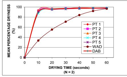
The Dyson Airblade hand dryer (DAB) had a drying efficiency equal to that of the 5 types of paper towel (PT 1 - PT 5) tested and, like them, achieved at least 90% dryness in 10 seconds. The warm air dryer (WAD) took an average of 47 seconds (over 4-times as long) to achieve 90% dryness, *i.e.* was slower than the Dyson Airblade dryer or the paper towels at drying the hands.
